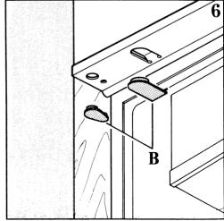
Depending on whether you have chosen left or right hand hinging, drill the appropriate holes in the fridge door and fix the appliance door runners (Fig. 7).
